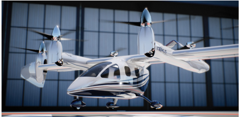
Developed by Textron eAviation, the Nexus eVTOL's 50-foot wingspan takes account of existing heliport design criteria and rotorcraft performance. Image: Textron eAviation
